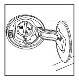
The tethered fuel cap is located behind a hinged fuel door on the passenger's side of the vehicle.
